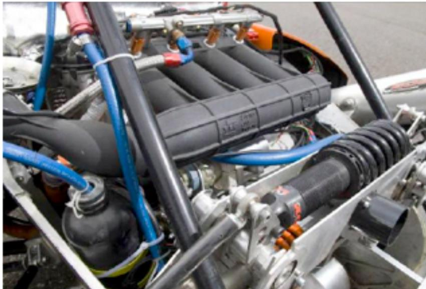
*Figure 1: Air intake manifold made using SLS at TNO, the Netherlands [11]*
